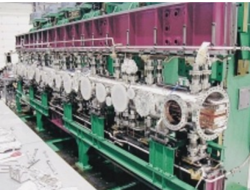
Spring8 IVUN (2000) Small gap In-vacuum device
