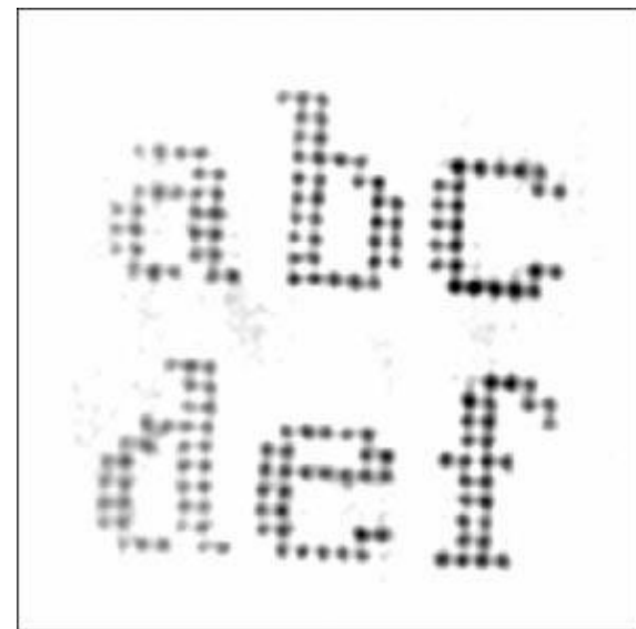
4- The specimen image as reconstructed from the diffraction pattern of Fig. 2.
